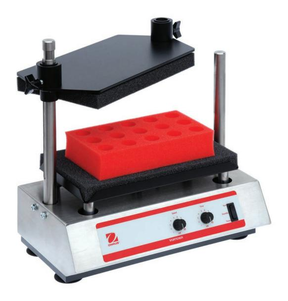
Multi-Tube Vortexers are ideal for high throughput sample processing. Interchangeable foam racks for vortexing tubes from 10 to 29 mm in diameter available. Vortexing action is created by securing the top of the sample in place while allowing the bottom to rotate freely in a 3.6 mm orbit. Suction cup feet reduce motion and prevent sliding on work surface. Analog & digital models, both microprocessor-controlled and run in continuous or timed mode.
